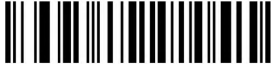
7 bit, 2 stop bit, no parity
